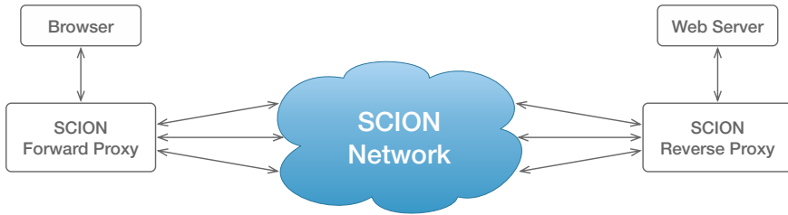
Figure 10.7: Deployment via SCION proxy.
